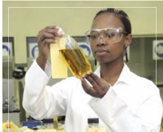
Khombi Ntshangase, Senior Lab Technician, checks the appearance of a sample of petrol for contamination.
