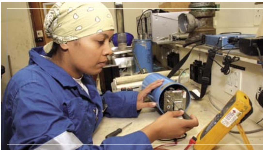
Felicia Alvar, Instrument Mechanic, tests a Flame Eye instrument in the workshop.
