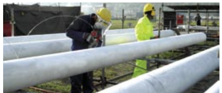
KAEFER Thermal applicator Cyprian Luthuli applies TSA coating to pipes while quality inspector Musa Ngidi conducts coating thickness checks.
